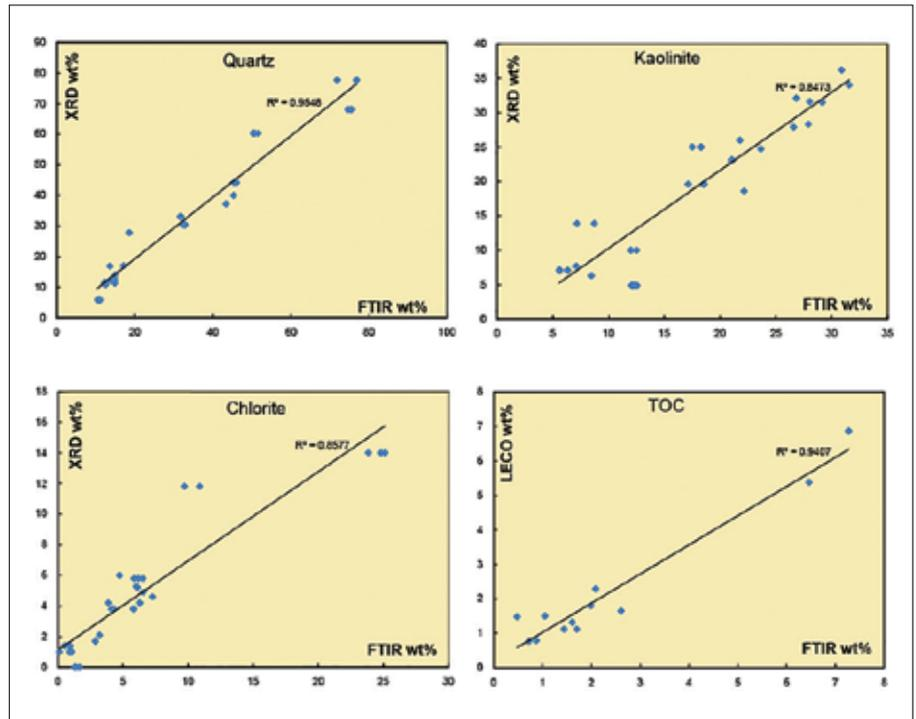
Fig. 3. Cross plots of selected variables obtained by XRD analysis (quartz, kaolinite, chlorite) and LECO analysis (TOC) compared against same variables obtained by FTIR analysis.
