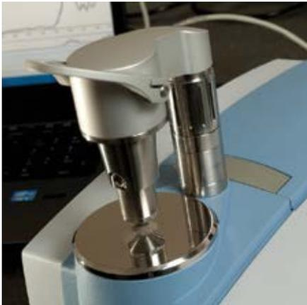
Fig. 4. Close up of instrument stage, with analysis underway. Note simple sample presentation protocol and small amount of sample required.
