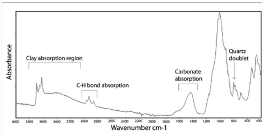
Fig. 1. FTiR absorbance spectrum showing the main peak associations with their mineralogical component. A range of clay minerals can be detected by the FTiR, this example shows predominantly kaolinite. A larger peak signifies a greater concentration of a component; however each peak has a different sensitivity to the component it shows.
