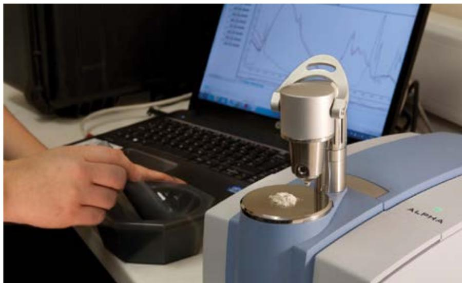
Fig. 2. The FTiR instrument is compact, lightweight and easy to use, pictured above is a powdered sample which is prepared in the pictured mortar and pestle.
